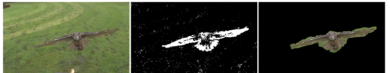
Figure 5: Motion Segmentation Example. Left : Original Frame. Middle : Thresholded Optical Flow Field. Right : Final Segmentation Results
